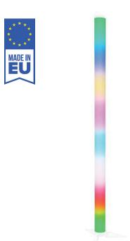
DIFFUSE TUBE RGB outdoor ambient luminaire with individual-pixel pitch 100mm step by SPI protocol. Special polycarbonate TUBE and UV stability-resistance and salt-mist proof. Gold plated PCB and use of HIGH quality RGB multichips NICHIA and constant current control inside the LED strip.
