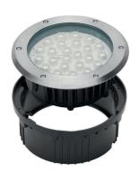
INGROUND 31 RGBW exterior luminaire with RGBW high-power OSRAM LED TECHNOLOGY. Passive cooling of LED with optimised heat sink geometry. No multiple shadows, energy-efficient LEDs with very good colour rendering.
